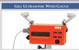
The Ultrasonic Wind Gauge is a key addition to the MVP package because it satisfies the I.A.A.F. and NFHS requirements for ratifying record-breaking times. In order for a new Track & Field record to be considered valid, it must be accompanied by a reading from a certified device that accurately measures head/tail winds during the race.
